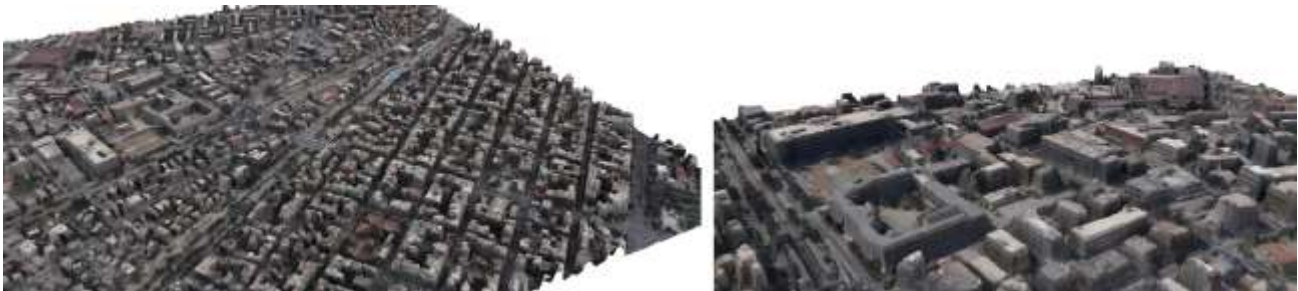
Figure 4. Texture mapping of the original Lidar surface from vertical and oblique aerial imagery.
