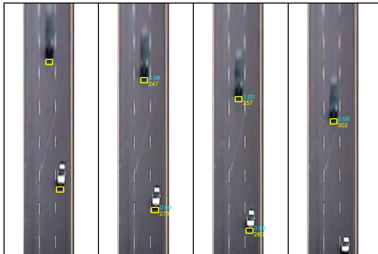
Figure 4. Tracking of detected profiles in three successive affine frames with cross-correlation.
