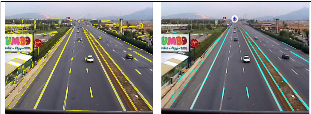
Figure 1. Left: extracted edges using the Canny detector. Right: automatic estimation of the vanishing point in the road direction.
