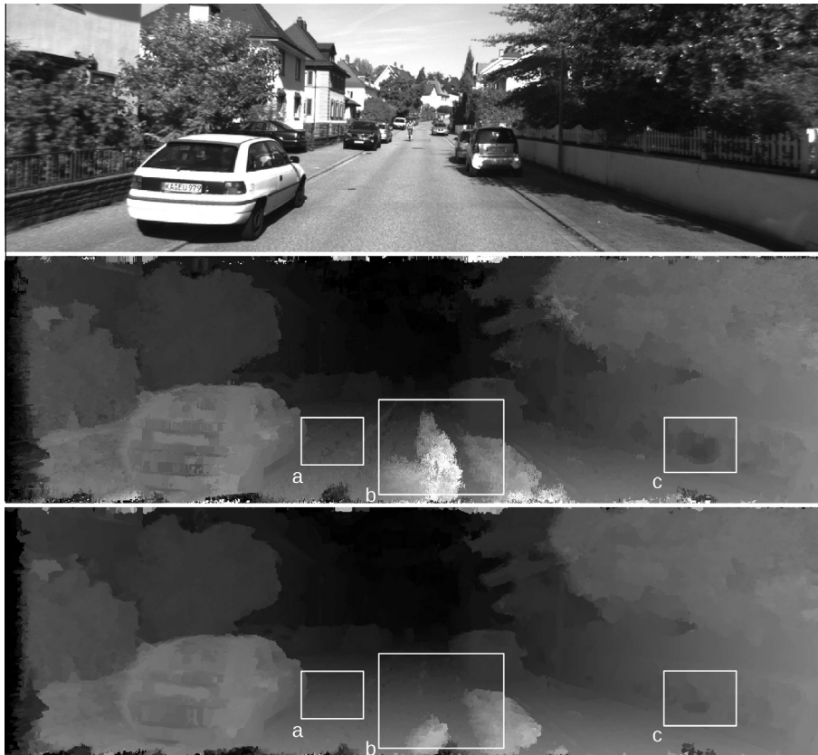
Fig. 10. Improvement of the disparity map through geometrically constrained smoothing of the cost function showing the estimated disparity map without (middle) and with (bottom) cost smoothing. Windows a , b and c indicate areas of improvement.
