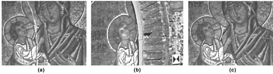
Figure 8. The artifact in the orthoimage detail (a) clearly originates from the occlusion border of the source image seen in (b). It has been filtered out in (c), where the corresponding detail of the final orthoimage (which is fully presented in Figure 9) is shown.
