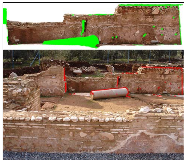
Figure 8. Orthoimage from one image (top) and projection of its occlusion borders onto the original image (bottom).
