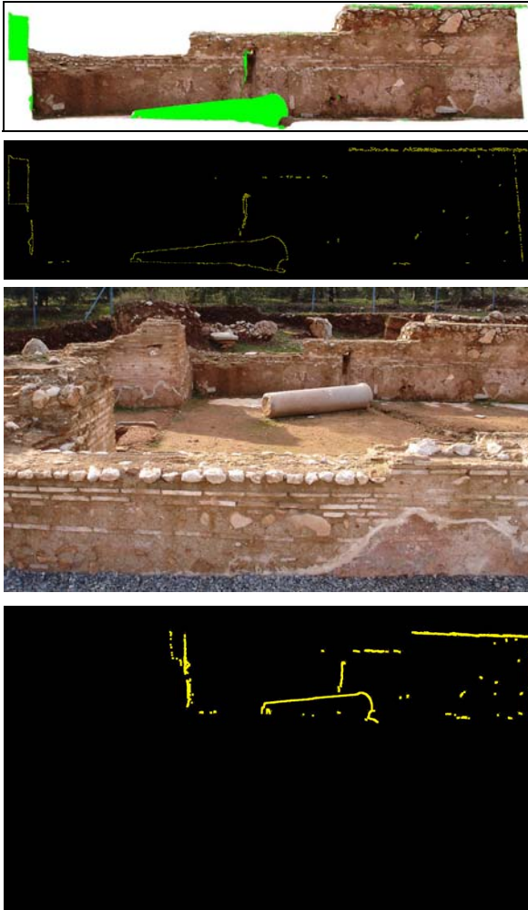
Figure 3. From top to bottom: orthoimage from a source image (image occluded areas in green); occlusion edges extracted after opening; original source image; orthoimage occlusion edges projected onto the source image and subjected to dilation.
